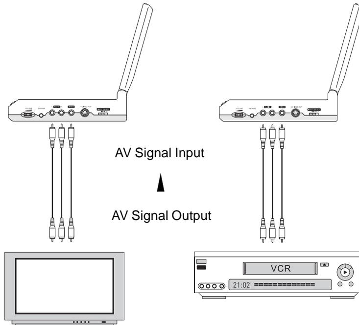
Your player is able to accept an AV signal input through the three AV jacks as soon as the **INPUT SELECT** switch has been switched to **IN**. Connecting the included or separately purchased AV cables into the player will permit input signals from at least the following types of peripherals:
